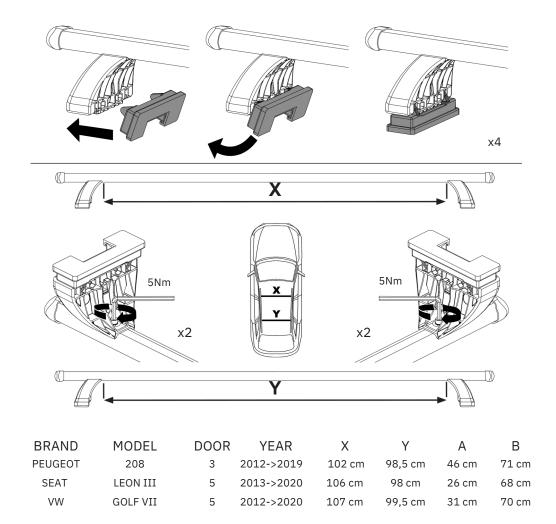
You must follow the measurements indicated in this table for your vehicle. Failure to follow these measurements will result in incorrect fitment of your roof bars, which will invalidate your warranty.
