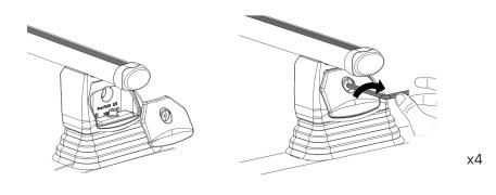
Inserting the lower rubber strip will reduce noise whilst driving.
