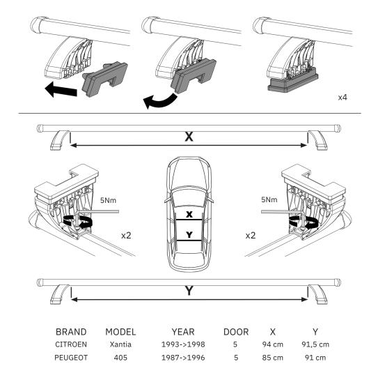
You must follow the measurements indicated in this table for your vehicle. Failure to follow these measurements will result in incorrect fitment of your roof bars, which will invalidate your warranty.
