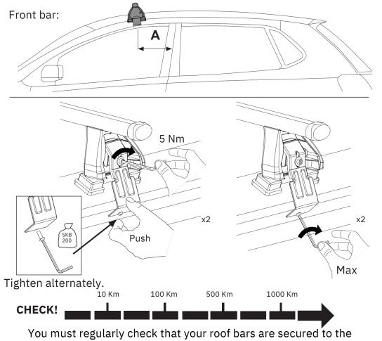
You must regularly check that your roof bars are secured to the correct Nm. We strongly recommend that you check & retighten your roof bars after the initial fitting, after adding & securing a load, before
