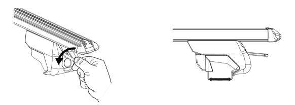
Ensure that the roof bars are parallel.
