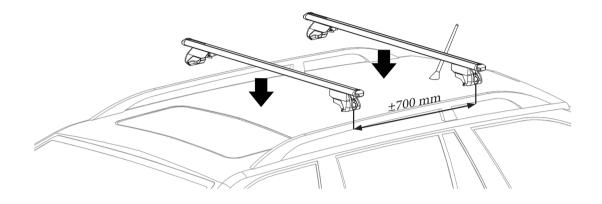
Ensure that the roof bars have even over hang on both sides.
