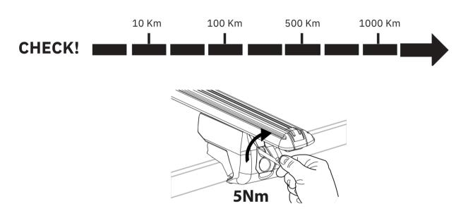
You must regularly check that your roof bars are secured to the correct Nm. We strongly recommend that you check & retighten your roof bars after the initial fitting, after adding & securing a load, before and during your journey.
