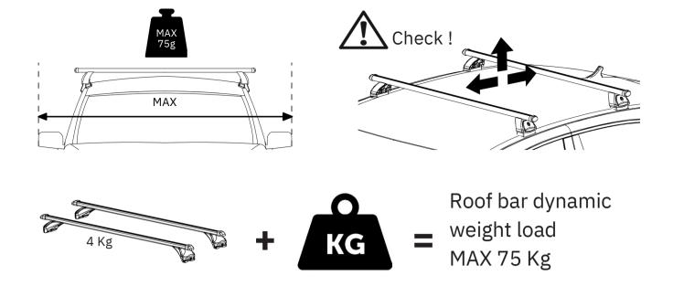
Check the vehicle handbook for the maximum permitted load. If the vehicle handbook states lower than 75kg, that must be observed, if more than 75kg the bar maximum dynamic weight must not be exceeded.
