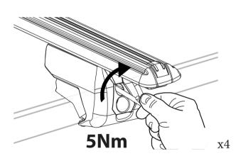
Tighten the feet alternately, to 5Nm.
