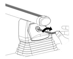
Tighten alternately, to 5Nm
