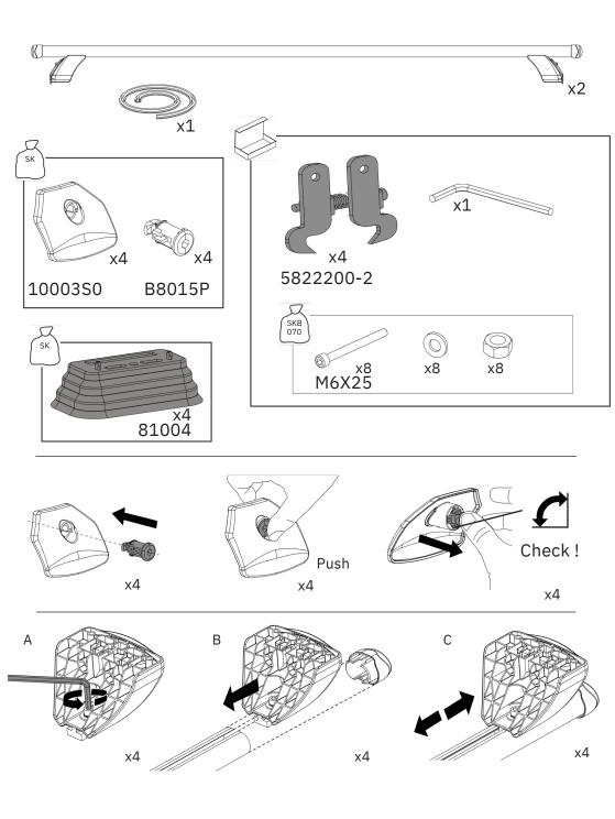
You will need to remove the mounting point covers. Ensure that the fix point mounting locations are clean & free from debris.
