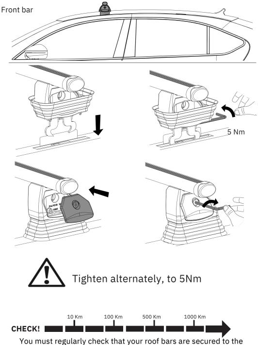
correct Nm. We strongly recommend that you check & retighten your roof bars after the initial fitting, after adding & securing a load, before and during your journey.
