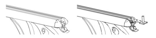
End cap can be opened to remove the rubber strip & insert T-Bolts for ease of adding accessories. You will need to cut the rubber strip to reinsert around the T-Bolts, and maintain the weatherproofing of the roof bars.
