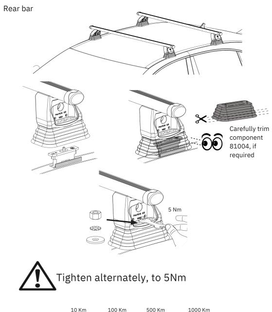
You must regularly check that your roof bars are secured to the correct Nm. We strongly recommend that you check & retighten your roof bars after the initial fitting, after adding & securing a load, before and during your journey.
