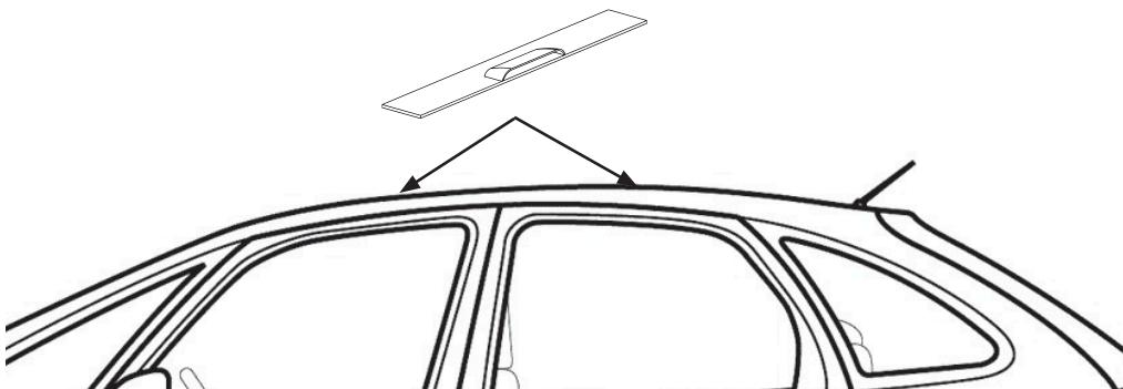
Front bar: Measure from the middle of the A pillar to the centre of the roof bar foot.
