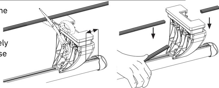
**X measurement:** Position of the feet on the front bar - you need the front of the feet to line up to this measurement.
