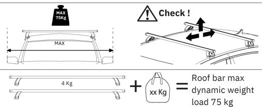
Check the vehicle handbook for the maximum permitted load. If the vehicle handbook states lower than 75kg, that must be observed, if more than 75kg the bar maximum dynamic weight must not be exceeded.
