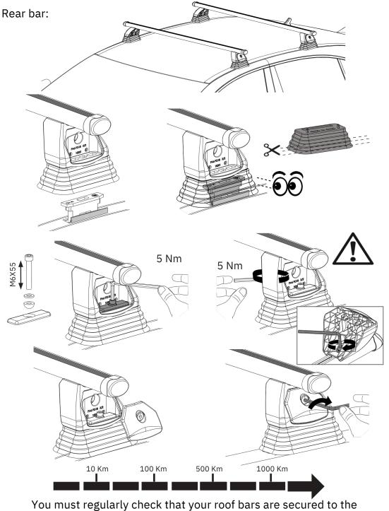
correct Nm. We strongly recommend that you check & retighten your roof bars after the initial fitting, after adding & securing a load, before and during your journey.
