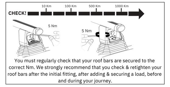
It is your responsibility to ensure that your roof bars & any roof load are correctly & securely fitted to your vehicle.
