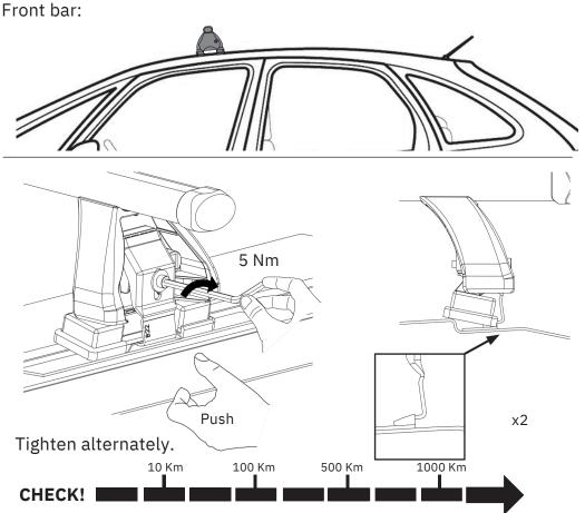
You must regularly check that your roof bars are secured to the correct Nm. We strongly recommend that you check & retighten your roof bars after the initial fitting, after adding & securing a load, before and during your journey.
