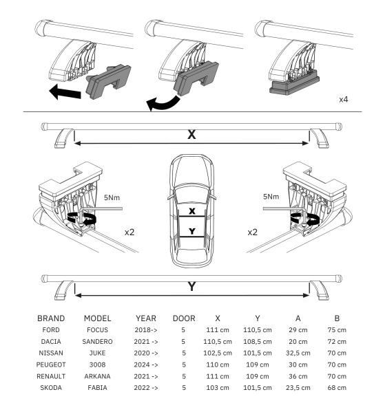
You must follow the measurements indicated in this table for your vehicle. Failure to follow these measurements will result in incorrect fitment of your roof bars, which will invalidate your warranty.
