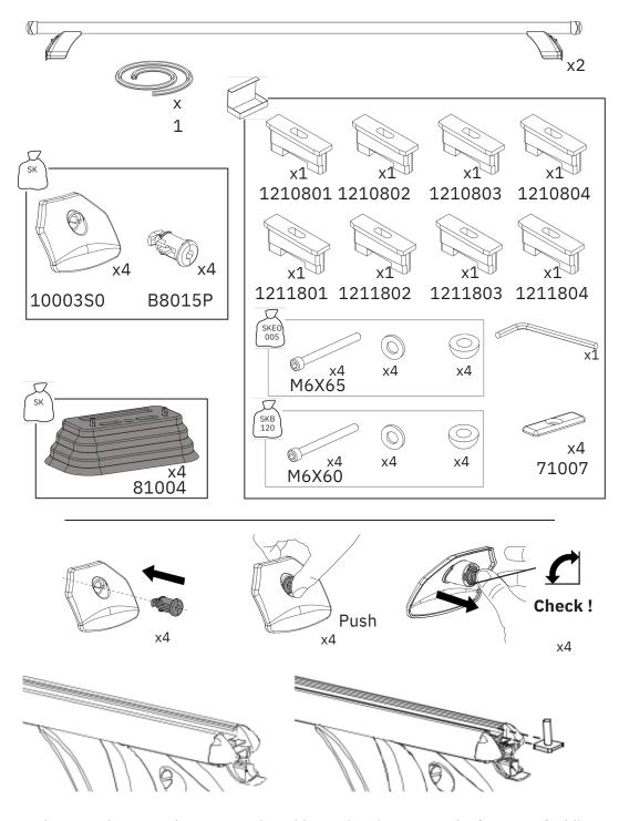
End cap can be opened to remove the rubber strip & insert T-Bolts for ease of adding accessories. You will need to cut the rubber strip to reinsert around the T-Bolts, and maintain the weatherproofing of the roof bars.
