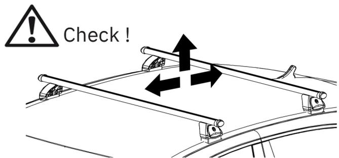
4 Kg + **KG** = Roof bar dynamic weight load MAX 75 Kg
