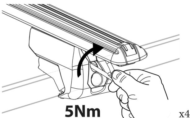
Tighten the feet alternately, to 5Nm.
