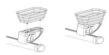
You must remove and cut any mounting cover trim. Your roof bars will not fit correctly if you do not follow this step!
