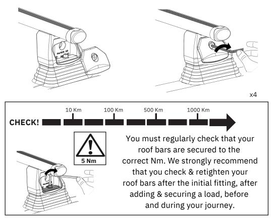
It is your responsibility to ensure that your roof bars & any roof load are correctly & securely fitted to your vehicle.
