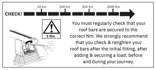
It is your responsibility to ensure that your roof bars & any roof load are correctly & securely fitted to your vehicle.
