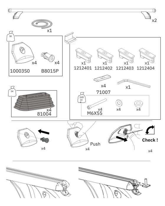
End cap can be opened to remove the rubber strip & insert T-Bolts for ease of adding accessories. You will need to cut the rubber strip to reinsert around the T-Bolts, and maintain the weatherproofing of the roof bars.
