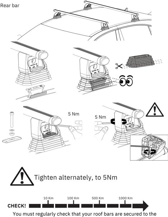
You must regularly check that your roof bars are secured to the correct Nm. We strongly recommend that you check & retighten your roof bars after the initial fitting, after adding & securing a load, before and during your journey.
