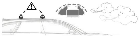
You must ensure that your fix point mounting locations are clean & free from debris, before you fit these roof bars.
