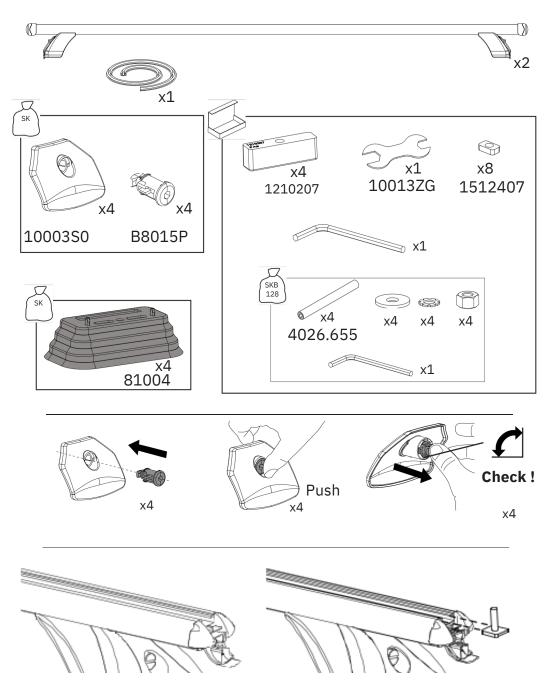
End cap can be opened to remove the rubber strip & insert T-Bolts for ease of adding accessories. You will need to cut the rubber strip to reinsert around the T-Bolts, and maintain the weatherproofing of the roof bars.
