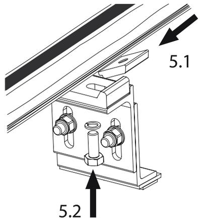
Place the bar onto the mounting brackets, insert the bar locator plate. Insert the 13mm headed bolt & washer from below, to hold in place.
