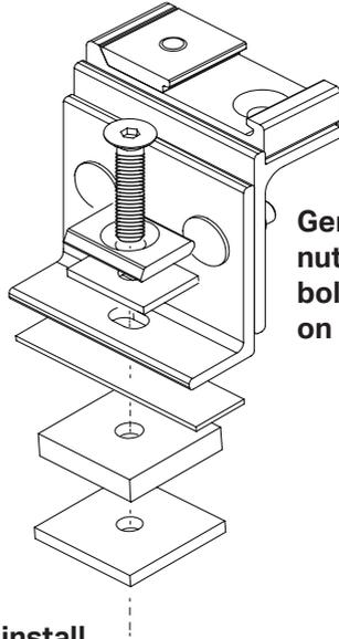
Gently tighten the nuts on the levelling bolts until they hold, on each bracket.
