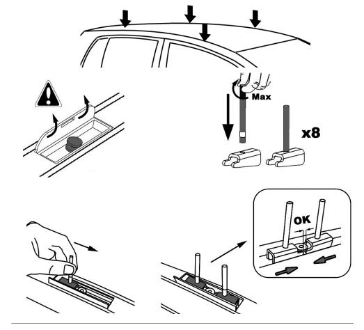
ONLY DS3 - REMOVE THE ROOF TRIM TO ACCESS MOUNTING POINTS.
