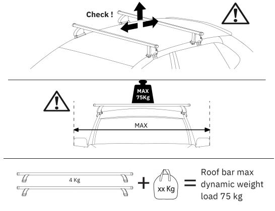
Check the vehicle handbook for the maximum permitted load. If the vehicle handbook states lower than 75kg, that must be observed, if more than 75kg the bar maximum dynamic weight must not be exceeded.
