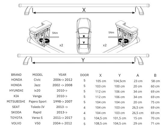
You must follow the measurements indicated in this table for your vehicle. Failure to follow these measurements will result in incorrect fitment of your roof bars, which will invalidate your warranty.
