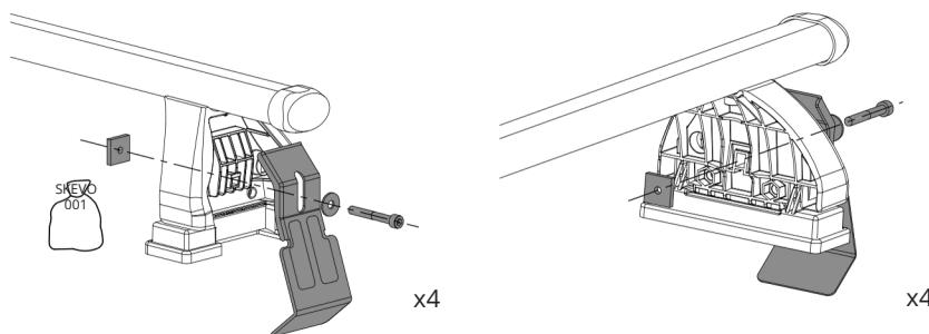
Front bar: Measure from the middle of the A pillar to the centre of the roof bar foot.
