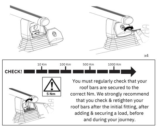
It is your responsibility to ensure that your roof bars & any roof load are correctly & securely fitted to your vehicle.
