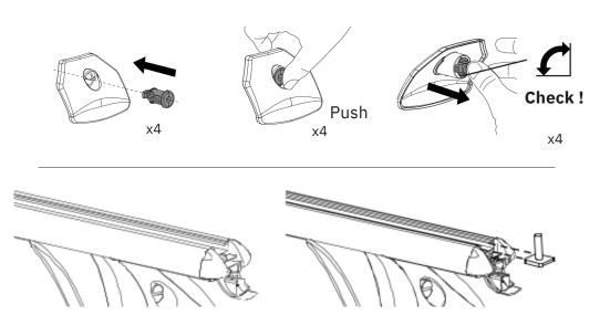
End cap can be opened to remove the rubber strip & insert T-Bolts for ease of adding accessories. You will need to cut the rubber strip to reinsert around the T-Bolts, and maintain the weatherproofing of the roof bars.
