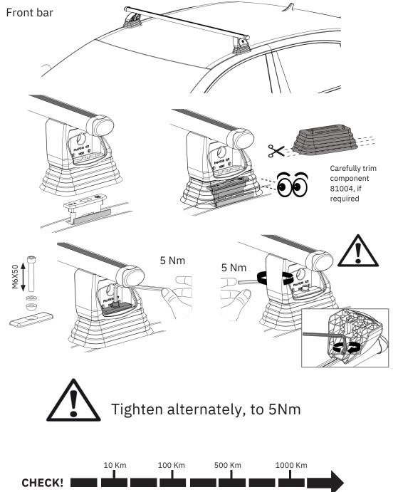
You must regularly check that your roof bars are secured to the correct Nm. We strongly recommend that you check & retighten your roof bars after the initial fitting, after adding & securing a load, before and during your journey.
