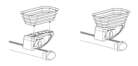
You must remove and cut any mounting cover trim. Your roof bars will not fit correctly if you do not follow this step!
