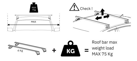
Check the vehicle handbook for the maximum permitted roof weight load. If the vehicle handbook states lower than 75kg, that must be observed, if more than 75kg the bar maximum dynamic weight must not be exceeded.
