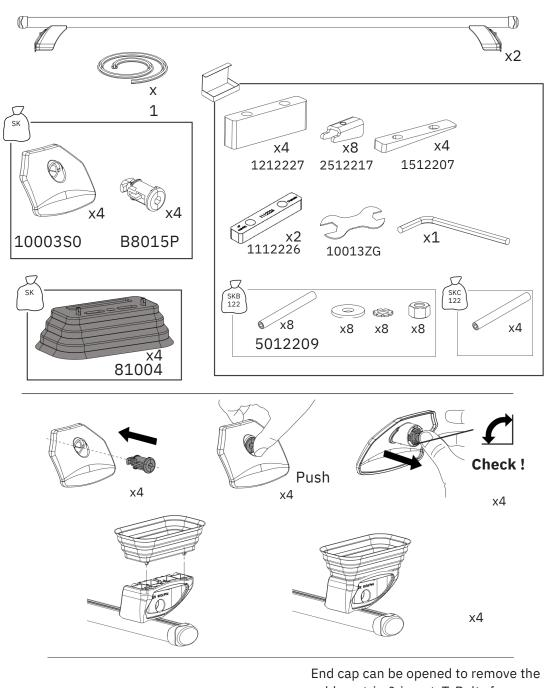
rubber strip & insert T-Bolts for ease of adding accessories. You will need to cut the rubber strip to reinsert around the T-Bolts, and maintain the weatherproofing of the roof bars.
