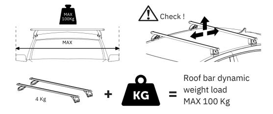
Check the vehicle handbook for the maximum permitted load. If the vehicle handbook states lower than 100kg, that must be observed, if more than 100kg the bar maximum dynamic weight must not be exceeded.
