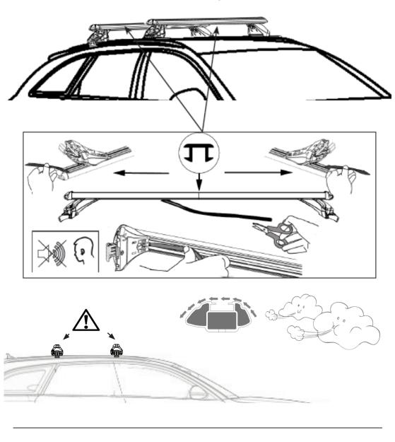
End cap can be opened to remove the rubber strip & insert T-Bolts for ease of adding accessories. You will need to cut the rubber strip to reinsert around the T-Bolts, to maintain the weatherproofing of the roof bars.
