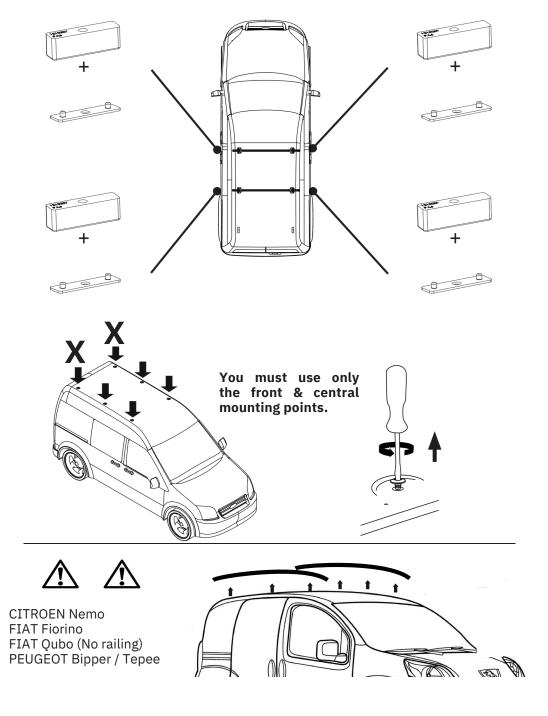
Remove the plastic covers (valid only for the models which are originally equipped with)
