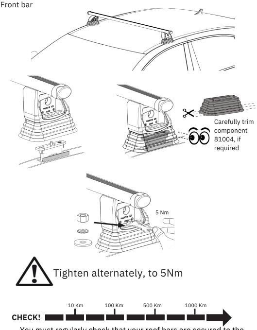
You must regularly check that your roof bars are secured to the correct Nm. We strongly recommend that you check & retighten your roof bars after the initial fitting, after adding & securing a load, before and during your journey. Rear bar
