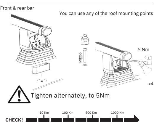
You must regularly check that your roof bars are secured to the correct Nm. We strongly recommend that you check & retighten your roof bars after the initial fitting, after adding & securing a load, before and during your journey.
