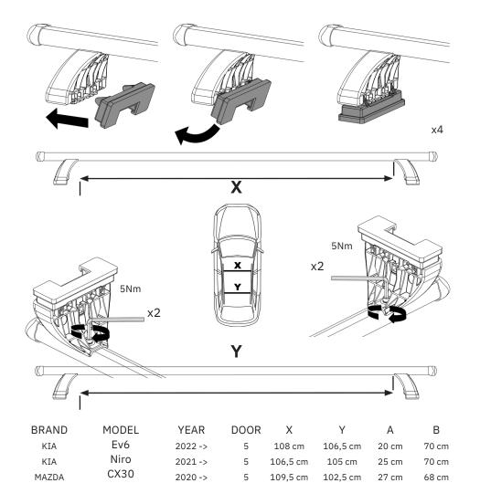
You must follow the measurements indicated in this table for your vehicle. Failure to follow these measurements will result in incorrect fitment of your roof bars, which will invalidate your warranty.
