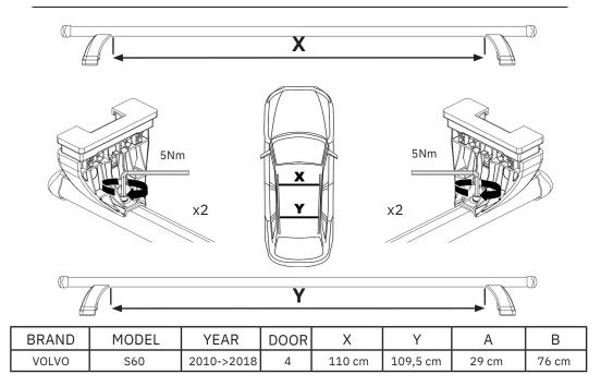
You must follow the measurements indicated in this table for your vehicle. Failure to follow these measurements will result in incorrect fitment of your roof bars, which will invalidate your warranty.
