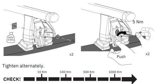
You must regularly check that your roof bars are secured to the correct Nm. We strongly recommend that you check & retighten your roof bars after the initial fitting, after adding & securing a load, before and during your journey.
