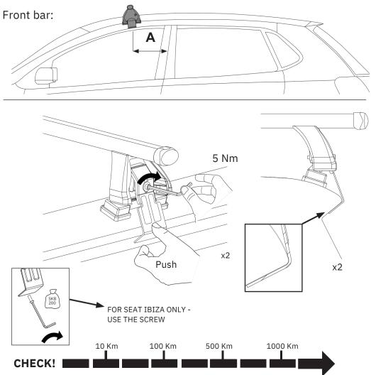
You must regularly check that your roof bars are secured to the correct Nm. We strongly recommend that you check & retighten your roof bars after the initial fitting, after adding & securing a load, before and during your journey.
