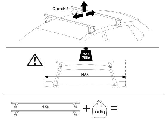
Check the vehicle handbook for the maximum permitted load. If the vehicle handbook states lower than 75kg, that must be observed, if more than 75kg the bar maximum dynamic weight must not be exceeded.
