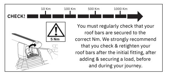
It is your responsibility to ensure that your roof bars & any roof load are correctly & securely fitted to your vehicle. Inserting the lower rubber strip will reduce noise whilst driving. After you have fitted your roof bars you can trim the rubber to size, as shown below.
