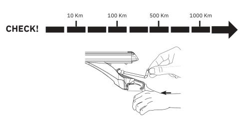
You must regularly check that your roof bars are secured to the correct Nm. We strongly recommend that you check & retighten your roof bars after the initial fitting, after adding & securing a load, before and during your journey.
