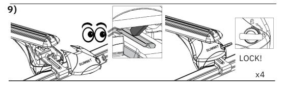
Insert the foot covers and lock them into place with the provided key.
