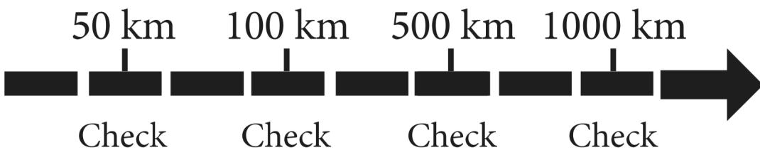
**You must regularly check that your roof bars are secured to the correct Nm. We strongly recommend that you check & retighten your roof bars after the initial fitting, after adding & securing a load, before and during your journey.**
