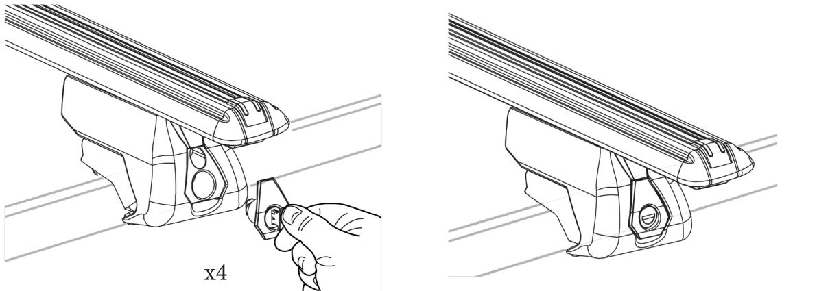
Trim the rubber strip to size and insert into the underneath roof bar cut-outs. This will reduce any noise from wind resistance.
