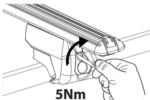
**You must regularly check that your roof bars are secured to the correct Nm. We strongly recommend that you check & retighten your roof bars after the initial fitting, after adding & securing a load, before and during your journey.**
