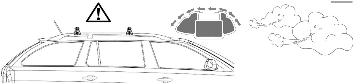
The roof bars must be fitted as per above, with the flatter edge forward. This ensures correct airflow, improves fuel economy and reduces noise.
