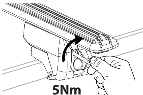
Tighten the feet alternately, to 5Nm.
