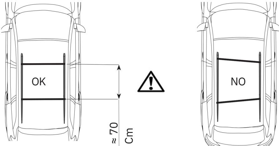
If the vehicle is equipped with original fix points, place the bars in the middle of them
