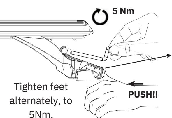
Tighten feet alternately, to 5Nm.
