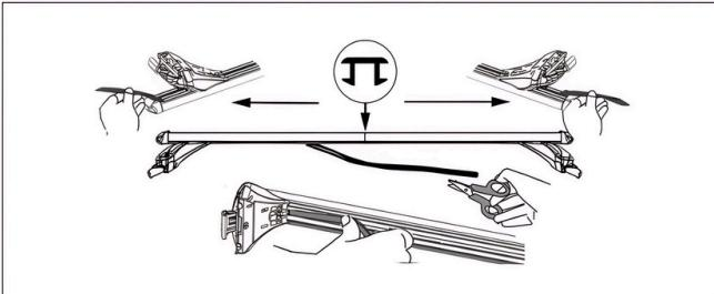
Trim the rubber strip to size and insert into the underneath roof bar cut-outs. This will reduce any noise from wind resistance.
