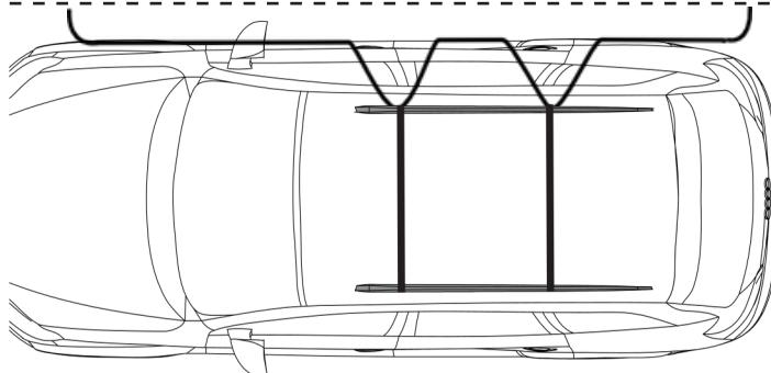
Ensure that the roof bars have even overhang on both sides.
