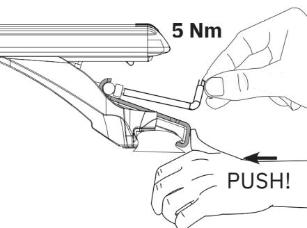
You must regularly check that your roof bars are secured to the correct Nm. We strongly recommend that you check & retighten your roof bars after the initial fitting, after adding & securing a load, before and during your journey.
