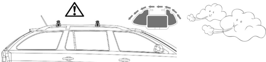
Ensure the roof bars are parallel.
