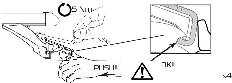
EN: Tighten your feet alternately on each side of the bar
