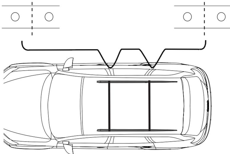
EN: If the vehicle is equipped with original fix points, place the bars in the middle of them
