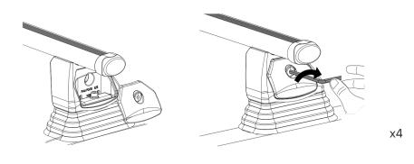
Inserting the lower rubber strip will reduce noise whilst driving.
