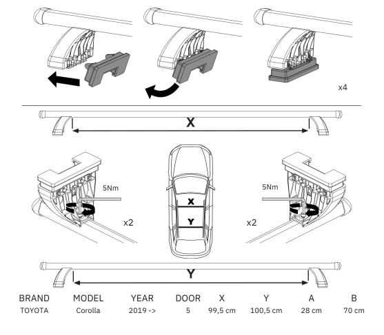
You must follow the measurements indicated in this table for your vehicle. Failure to follow these measurements will result in incorrect fitment of your roof bars, which will invalidate your warranty.
