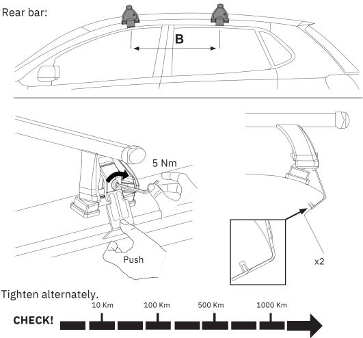
You must regularly check that your roof bars are secured to the correct Nm. We strongly recommend that you check & retighten your roof bars after the initial fitting, after adding & securing a load, before and during your journey.
