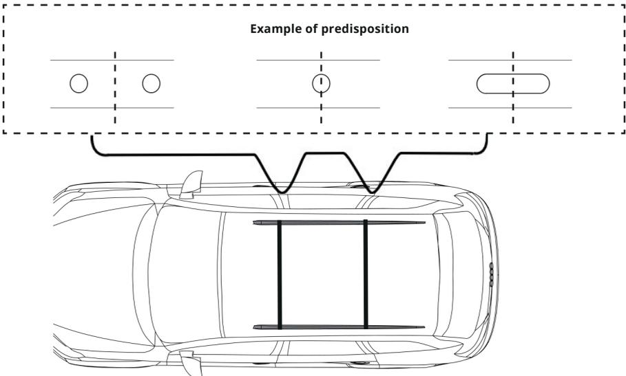
If the vehicle is equipped with original fix points, place the bars in the middle of them
