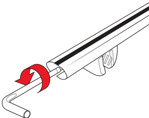
Using the Allen key provided, fully open the clamp mechanism inside the roof bars, this mechanism tightens the foot clamp onto the bar & also onto the roof bars themselves.
