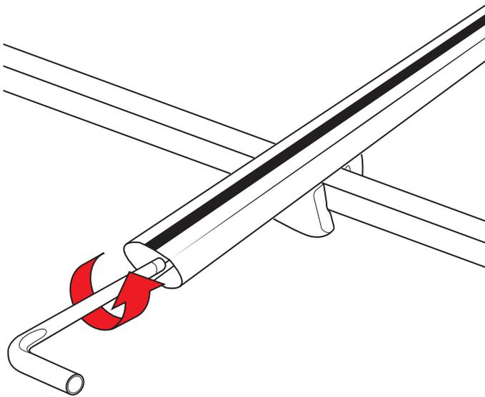
Using the Allen key, tighten the foot clamps **alternately** onto each side of the roof bar.
