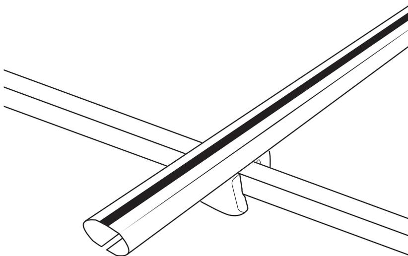
Place the roof bars onto the vehicles original rails, ensuring the positional guidance in step 2 is followed.
