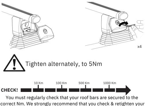
roof bars after the initial fitting, after adding & securing a load, before and during your journey.
