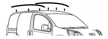
Remove the plastic covers (valid only for the models which are originally equipped with)
