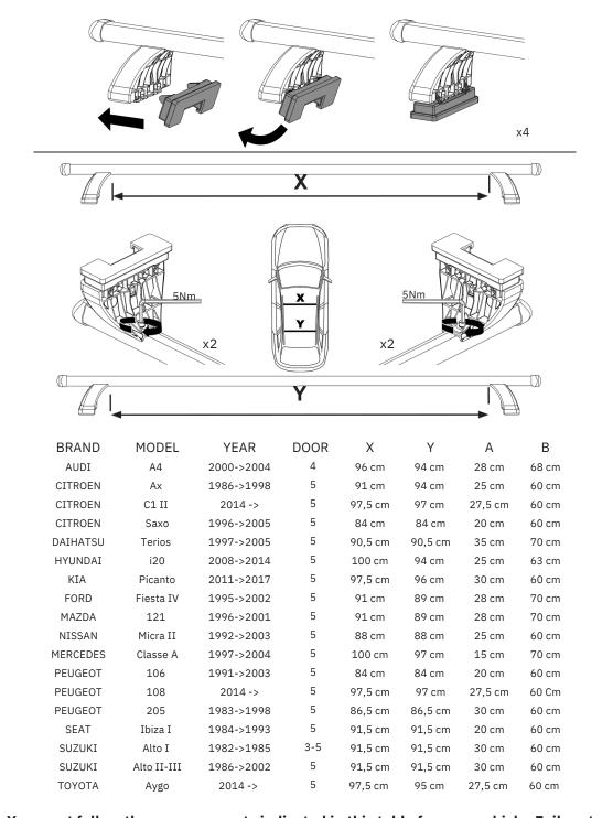
You must follow the measurements indicated in this table for your vehicle. Failure to follow these measurements will result in incorrect fitment of your roof bars, which will invalidate your warranty.
