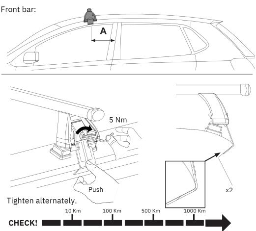
You must regularly check that your roof bars are secured to the correct Nm. We strongly recommend that you check & retighten your roof bars after the initial fitting, after adding & securing a load, before and during your journey.
