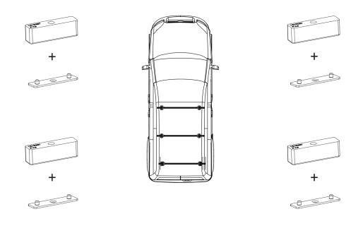
You may need to remove the vehicles mounting point covers. Only remove the covers where you will be placing the roof bars
