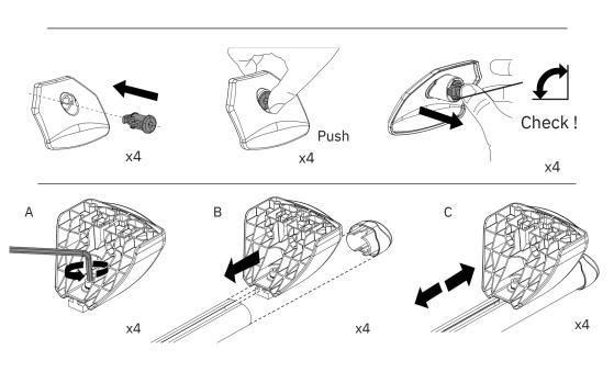
You will need to remove the mounting point covers. Ensure that the fix point mounting locations are clean & free from debris.
