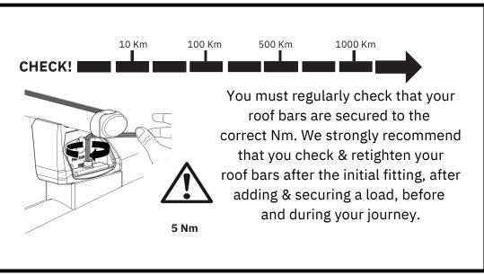
It is your responsibility to ensure that your roof bars & any roof load are correctly & securely fitted to your vehicle.
