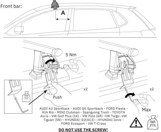
Tighten alternately. 100 Km 500 Km 1000 Km CHECK!
