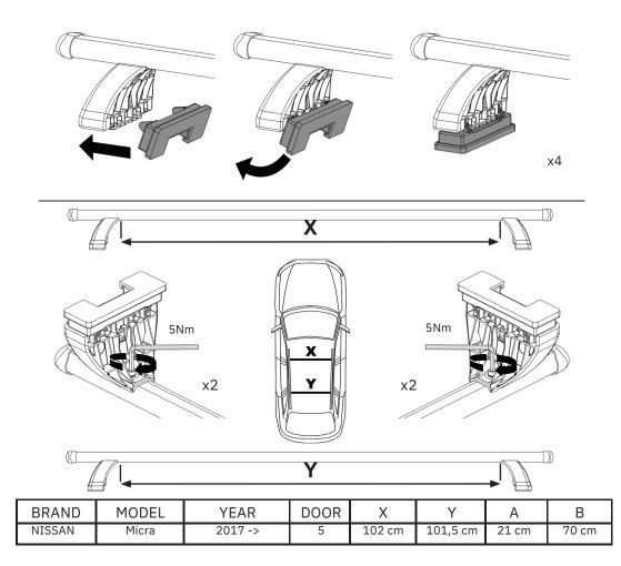
You must follow the measurements indicated in this table for your vehicle. Failure to follow these measurements will result in incorrect fitment of your roof bars, which will invalidate your warranty.
