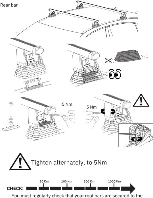
roof bars after the initial fitting, after adding & securing a load, before and during your journey.
