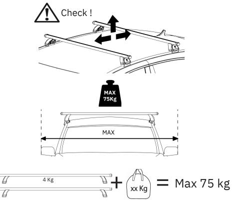
Check the vehicle handbook for the maximum permitted load. If the vehicle handbook states lower than 75kg, that must be observed, if more than 75kg the bar maximum dynamic weight must not be exceeded.
