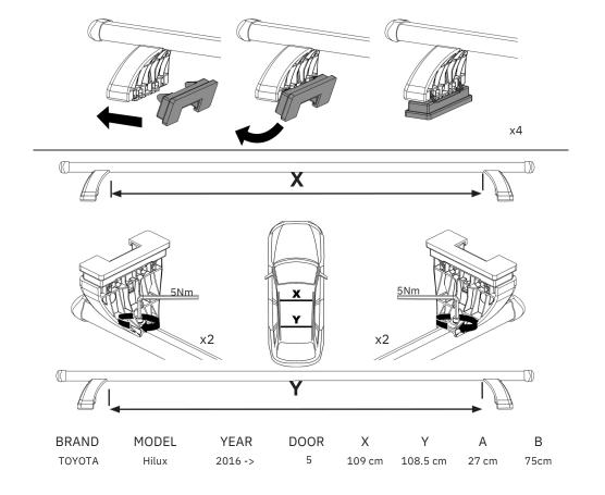
You must follow the measurements indicated in this table for your vehicle. Failure to follow these measurements will result in incorrect fitment of your roof bars, which will invalidate your warranty.
